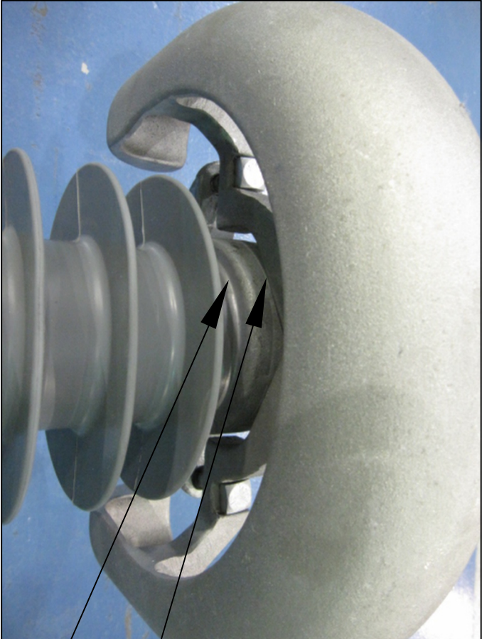
Edge of mounting arm is approx. 1/2"-1" from metal / rubber interface
