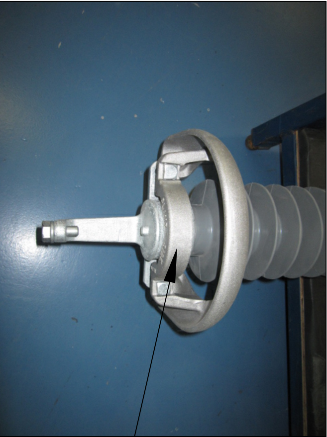
The Mounting arm fits onto the space between the lip and the step of the end fitting
