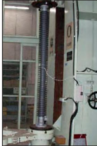
Torsion Strength Test
