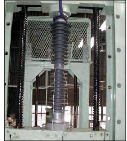
Compression Strength Test
