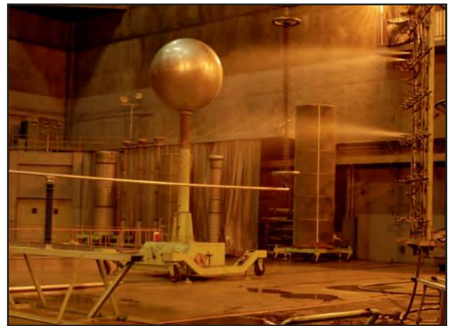
Low-Frequency Wet Withstand Test
